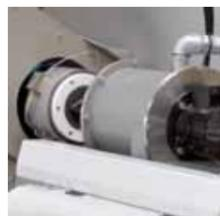
The patented water ring pelletiser ensures exact cutting for increased pellet quality and reduced wear of knives. Alternatively, strand, automatic strand, or underwater pelletising can be used.
