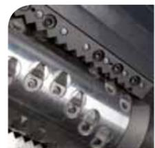
The hydraulic pusher in the single-shaft cutter presses the material against the water-cooled rotating shaft and thus ensures efficient crushing. The extruder-controlled dosing screw allows continuous feeding of the extruder even when the bulk density varies.
