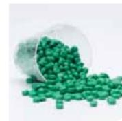
**The high pellet quality** ensures the production of an end-product with the characteristics of the original product. Up to 100 % reuse is possible. Additives can be added to increase the possibilities of reuse by adjusting pellet characteristics.
