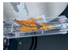
Optimally prepared material is fed by centrifugal force continuously into the extruder; overloading and underloading are avoided by load-control.
