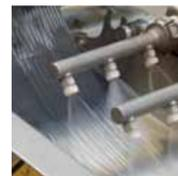
**The pelletising solutions** are chosen depending on polymer type and preferred pellet shape. In case of automatic strand pelletising, broken strands are automatically inserted into the strand pelletiser without operator interference. Alternatively, manual strand, water ring, or underwater pelletising are available.
