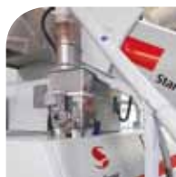
Powder dosing unit with special design to avoid bridging.
