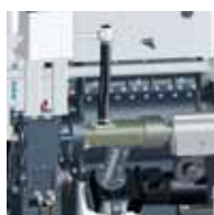
Separate powder and recycling material dosing ensures a constant ratio.
