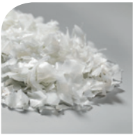
HDPE flakes are heated and dried, which forms the first decontamination step.
